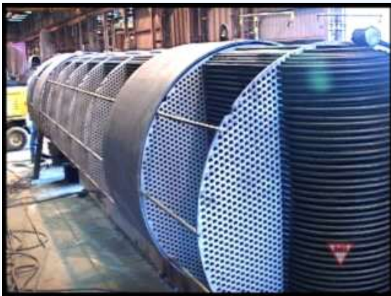
Plate Baffle Example
