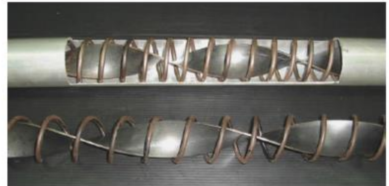
Fig. 10. Tube having twisted tape inserts and wire coil [28].
