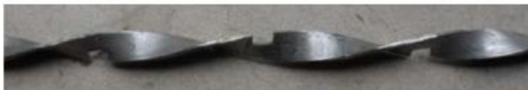
Fig. 22. rectangular cut twisted tape tested [48].
