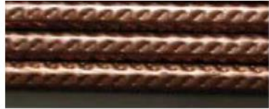
Fig. 17. Photo of the novel enhanced heat transfer tube [24].
