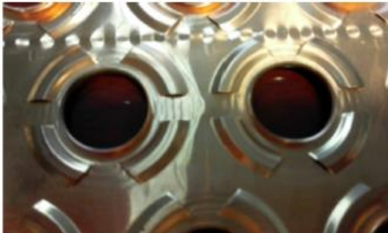
(b) Magnified picture of the four convex-strips around tube
