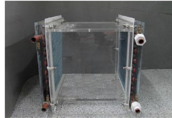
(b) Photo of the mixing device placed amid the first and the second heat exchanger.
