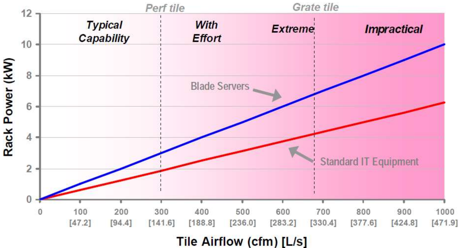
Figure 3 – Available rack enclosure cooling capacity of a floor tile as a function of per-tile airflow
