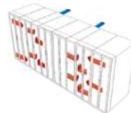
Targeted supply and contained return with cooling units located in the row
