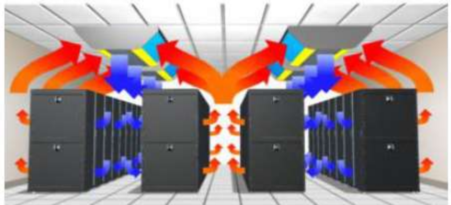
Figure 2b – Overhead cooling solution
